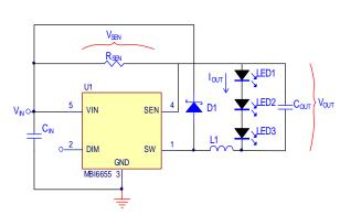
Figure 1. Application circuit of MBI6655
